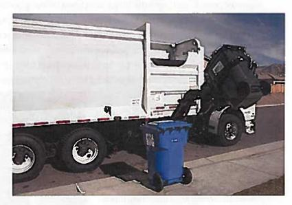
contents into the vehicle. The driver then uses the arm to return the container to its original location. The entire collection route can be serviced by the driver. This eliminates the manual labor that leads to frequent injuries, employee turnover as well as extra costs. Additionally crew productivity is increased. An automated system will allow the City to make twice as many stops in a day with one-third the manpower.
