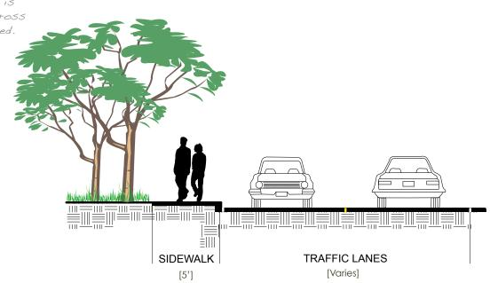
Right: Where space and topography are limiting and a planted buffer is not possible, this cross section may be applied.
