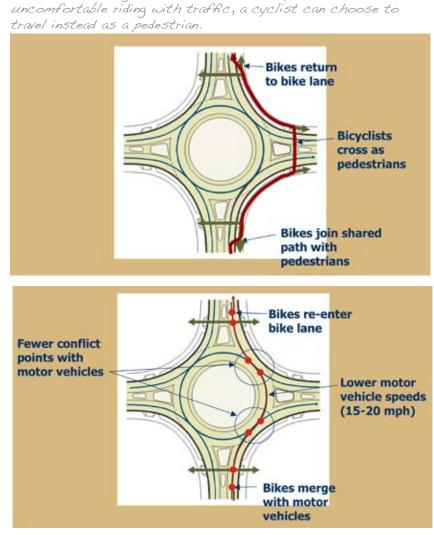
Above: Circulating as a Vehicle: Bike lanes are not recommended within a roundabout. Instead, cyclists merge with traffic before entering the roundabout, circulate with traffic, and then re-enter the bike lane after existing.
