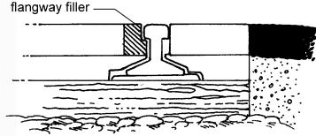
The "flangeway filler" eliminates the gap in the path of travel for pedestrians crossing railroad tracks. The filler, consisting of a rubber insert, will deflect downward with the weight of a train and does not affect railway function.
