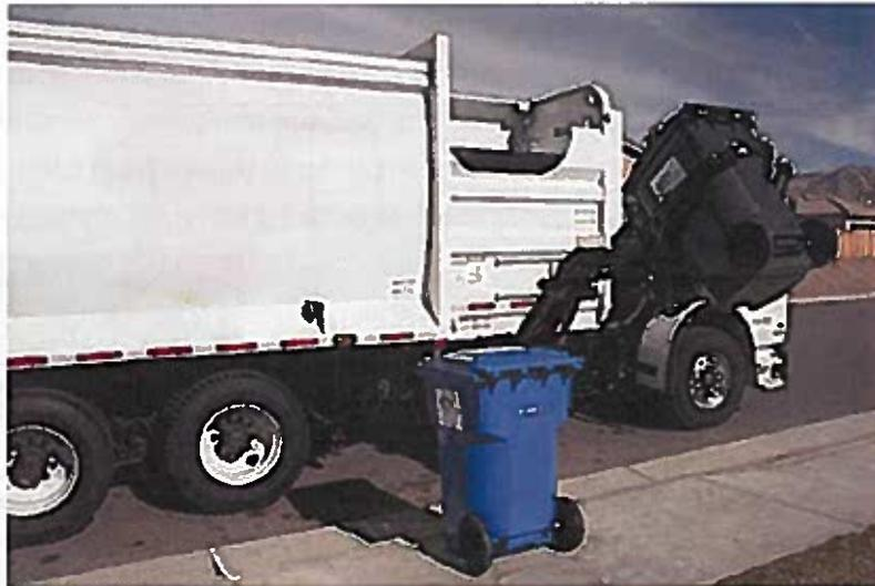
contents into the vehicle. The driver then uses the arm to return the container to its original location. The entire collection route can be serviced by the driver. This eliminates the manual labor that leads to frequent injuries, employee turnover as well as extra costs. Additionally crew productivity is increased. An automated system will allow the City to make twice as many stops in a day with one-third the manpower.
