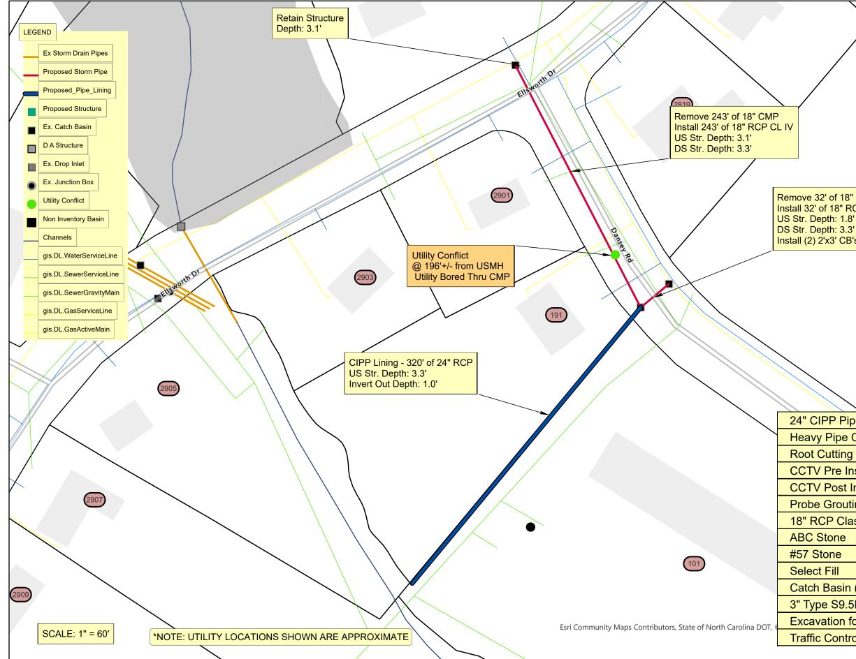
Remove 32' of 18" CMP Install 32' of 18" RCP CL IV US Str. Depth: 1.8' DS Str. Depth: 3.3' Install (2) 2'x3' CB's w/ Hood, Grate & Frame
