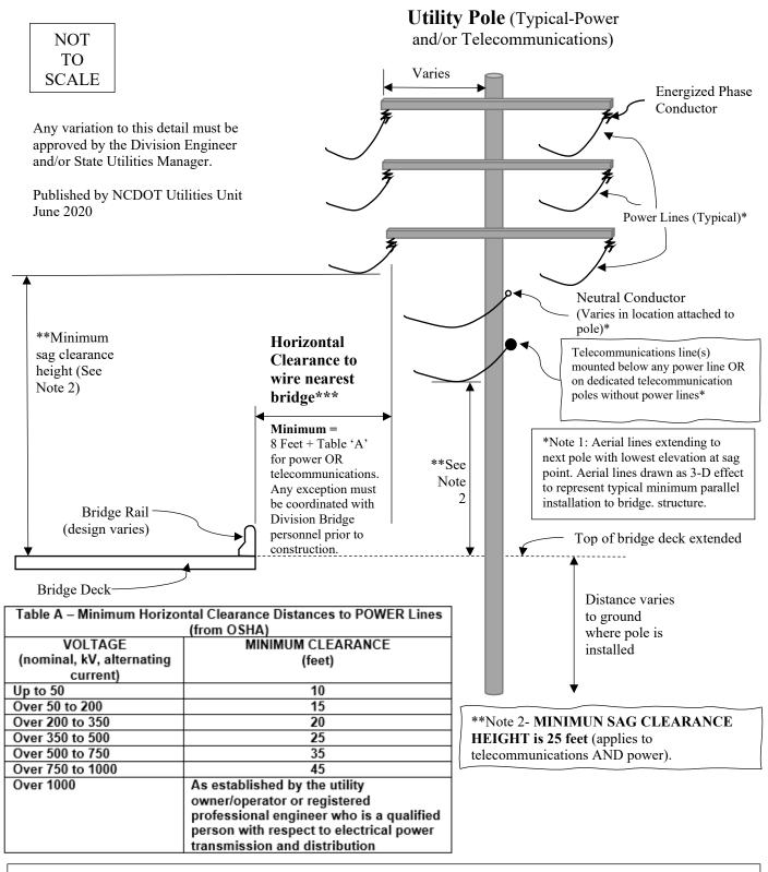
\*\*\*Note 3: HORIZONTAL CLEARANCE EXCEPTION. If vertical sag clearance height for power above bridge deck is  $\geq$  45 feet AND voltage is  $\leq$  350kV, then Minimum Horizontal Clearance may be reduced to 3 feet. Any telecommunications attachment to power pole allowed in this exception must have a minimum 25 feet sag clearance height above bridge deck.
