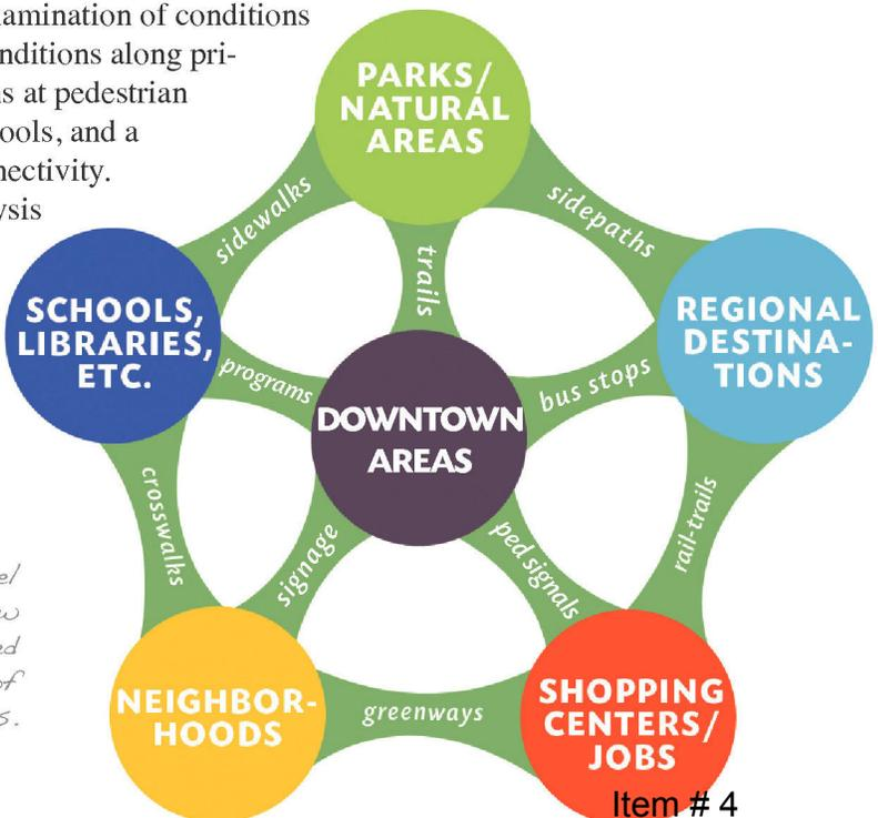
*The 'hubs and spokes' model conceptually illustrates how key destinations can be linked through various types of pedestrian facilities.*
